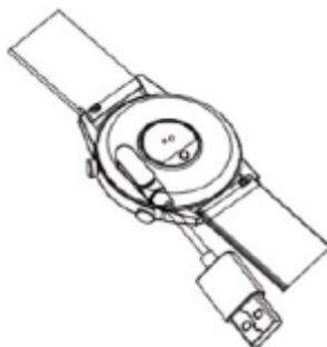
Connect and charge the watch according to the picture. It needs to be charged to activate the watch when it is started for the first time.
