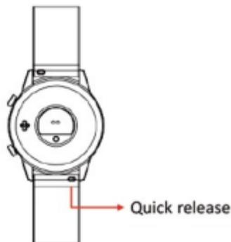
Remove the strap from the watch by sliding the quick release on the strap.
